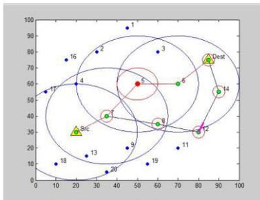
Fig: 11 Alternate Path from Source and Destination
